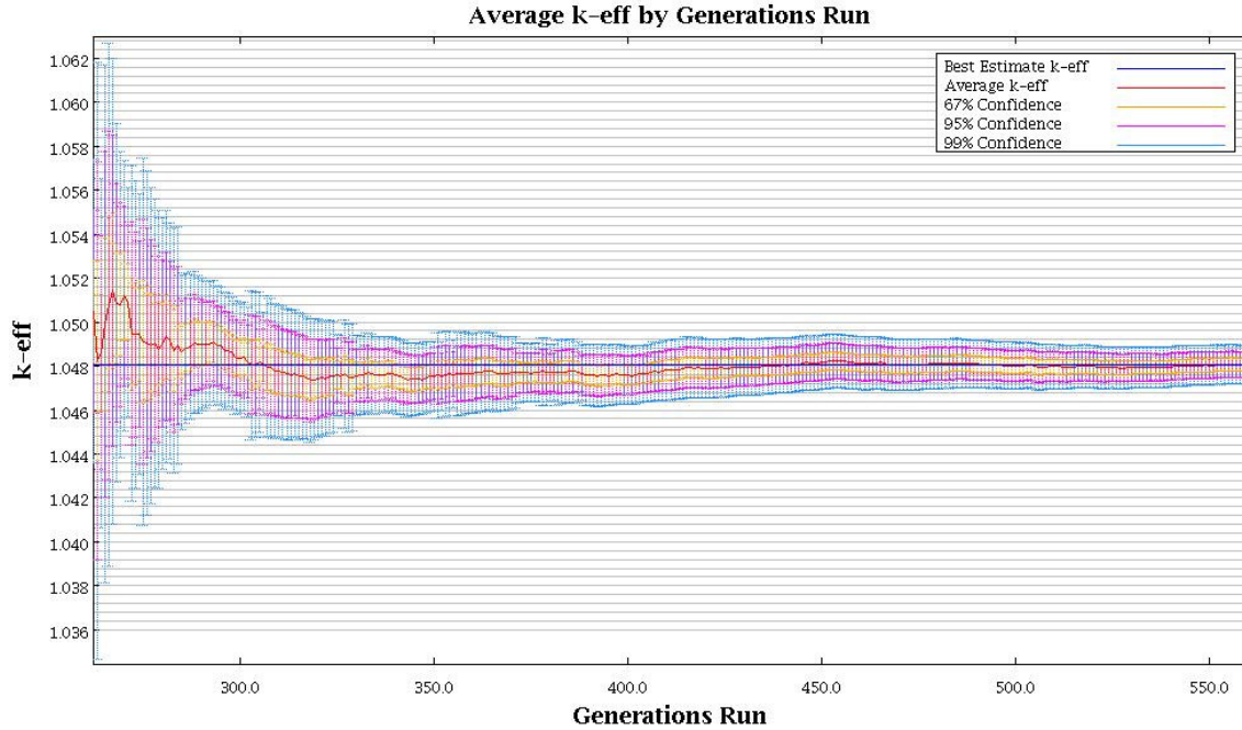
Figure 4.6: Average k-effective value by the number of generation run at end of reactor period.
